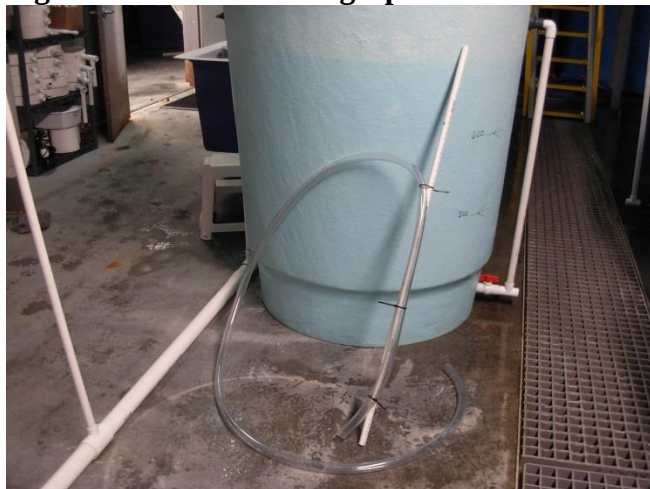
Figure 23. Tank cleaning siphon.
