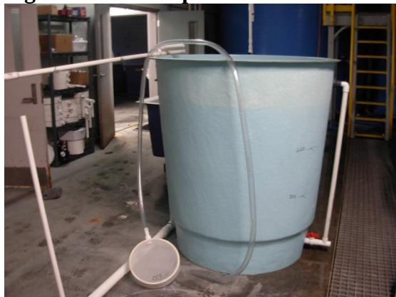
Figure 24. LRT siphon sieve.
